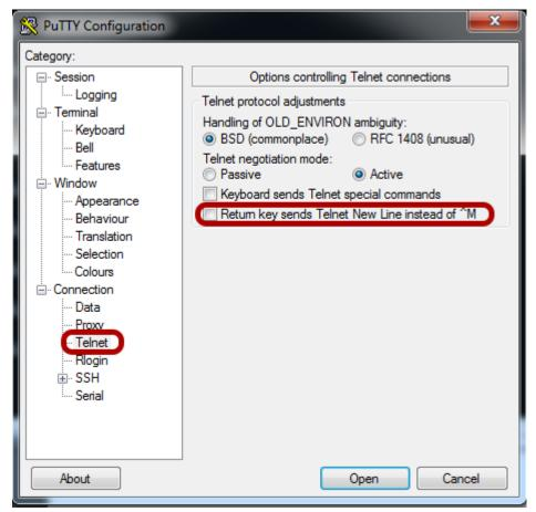
The default configuration under Connection > Telnet has also to be changed. Untick ""Return key sends Telnet New Line instead of  $^M$ ""
