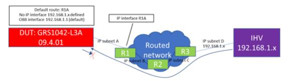
The GRS was configured correctly with a default route pointing to the next interface of router R1. Default IP address is configured for the OOB interface (192.168.1.1) and no changes were made for this interface.
